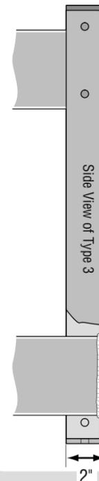
**⚠ Weld *Completely* around posts**
